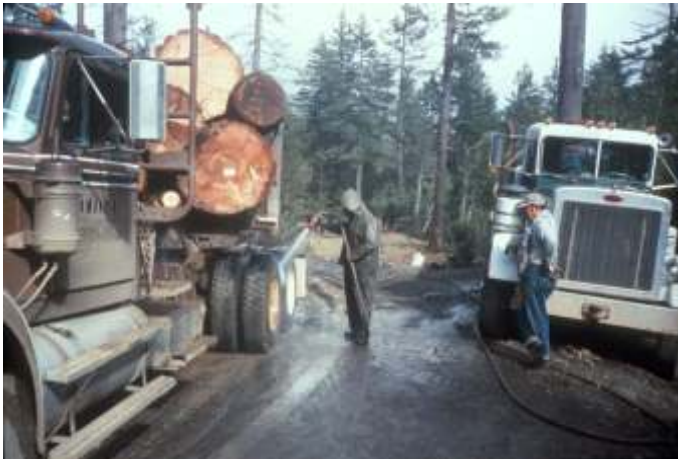
Figure 9. Washing of vehicle leaving infested site.
